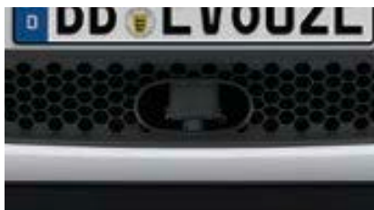
Radarsensor (Aktiver Brems-Assistent) [258]
